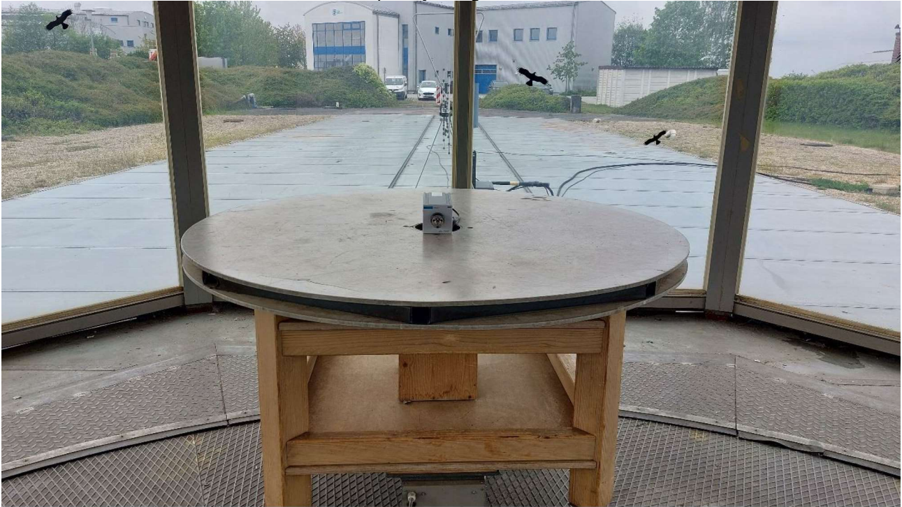
OATS 1 – Frequency Range: 30 MHz to 1 GHz
