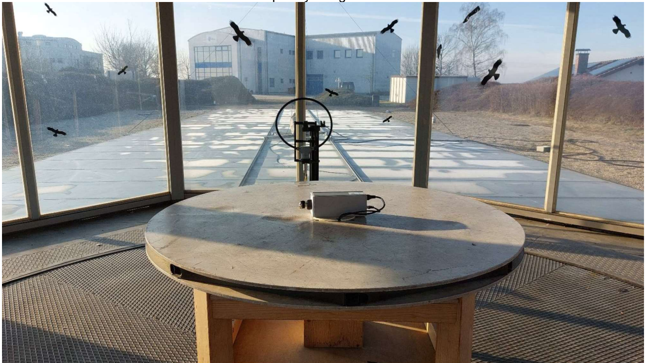
OATS 1 – Frequency Range: 9 kHz to 30 MHz
