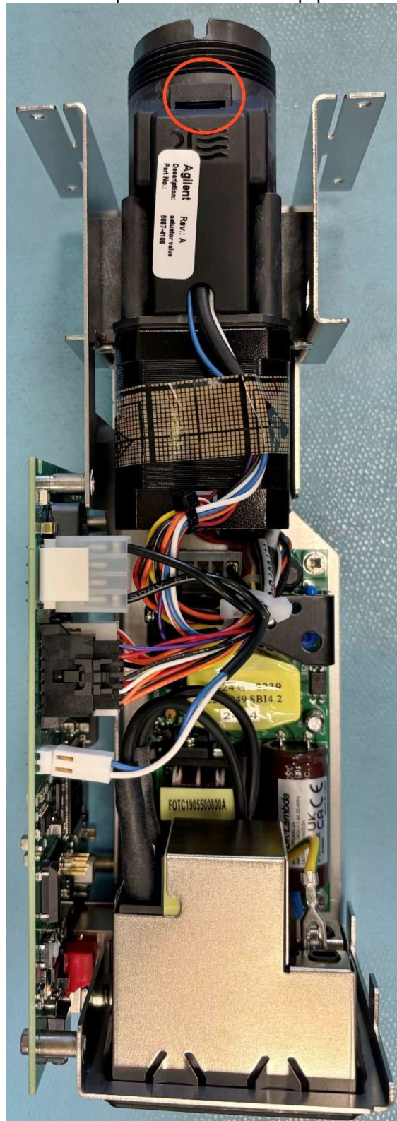
Antenna positions inside the equipment
