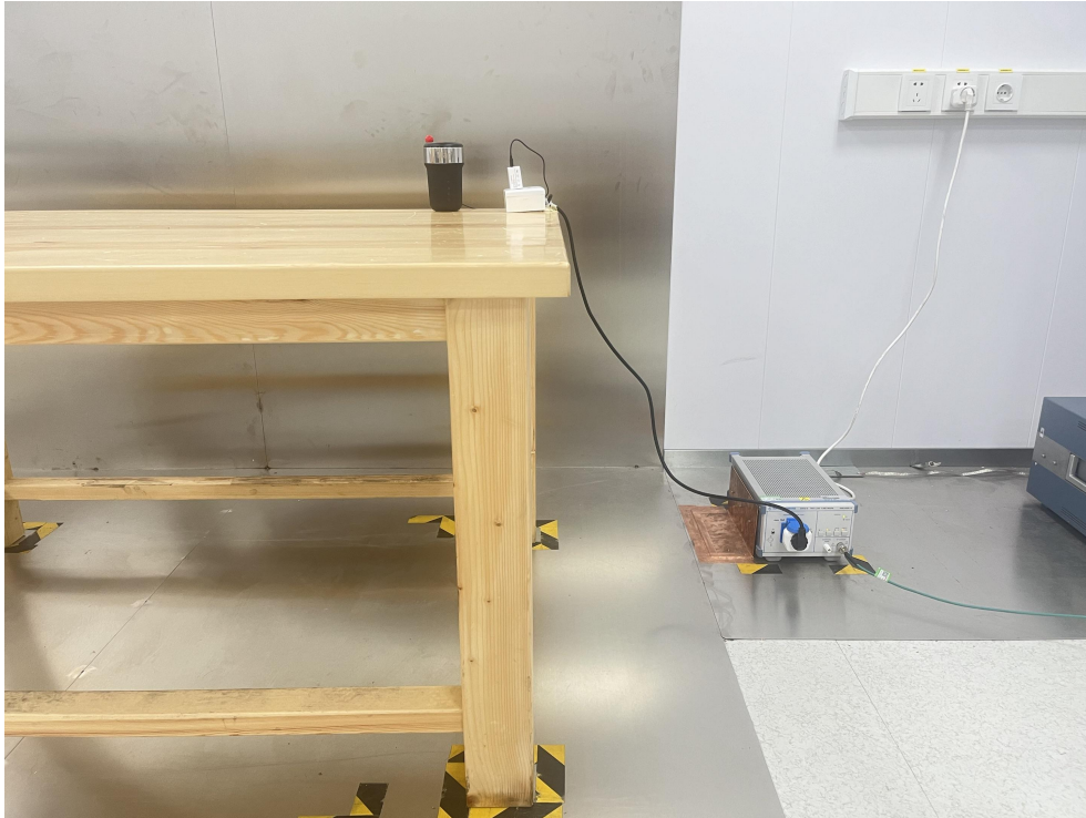
Radiated Emission Test View|(Below 1G)
