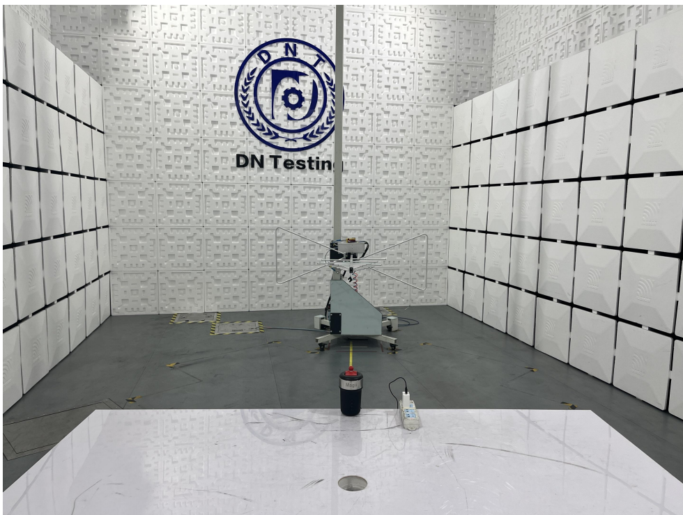
Radiated Emission Test View|(Below 1G)
