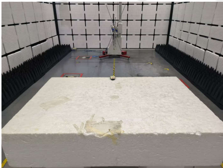
Radiated spurious emission Test Setup-1(Below 1GHz)
