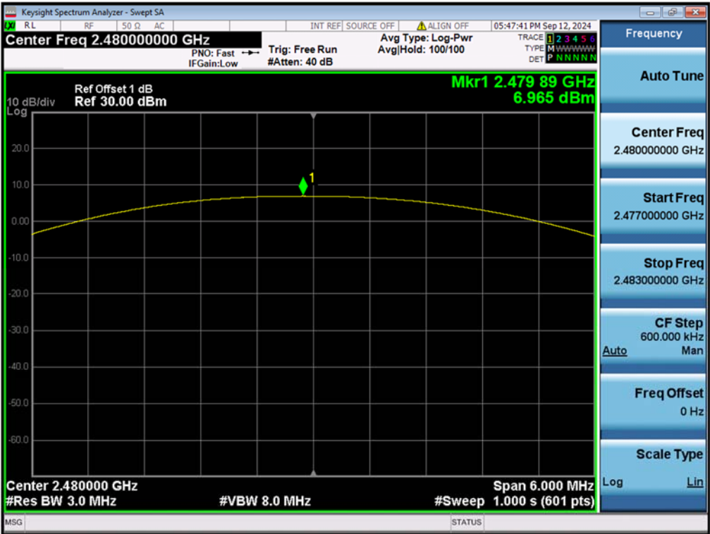
Figure 6: Maximum Peak Output Power, 2480MHz, \pi/4 -DQPSK
