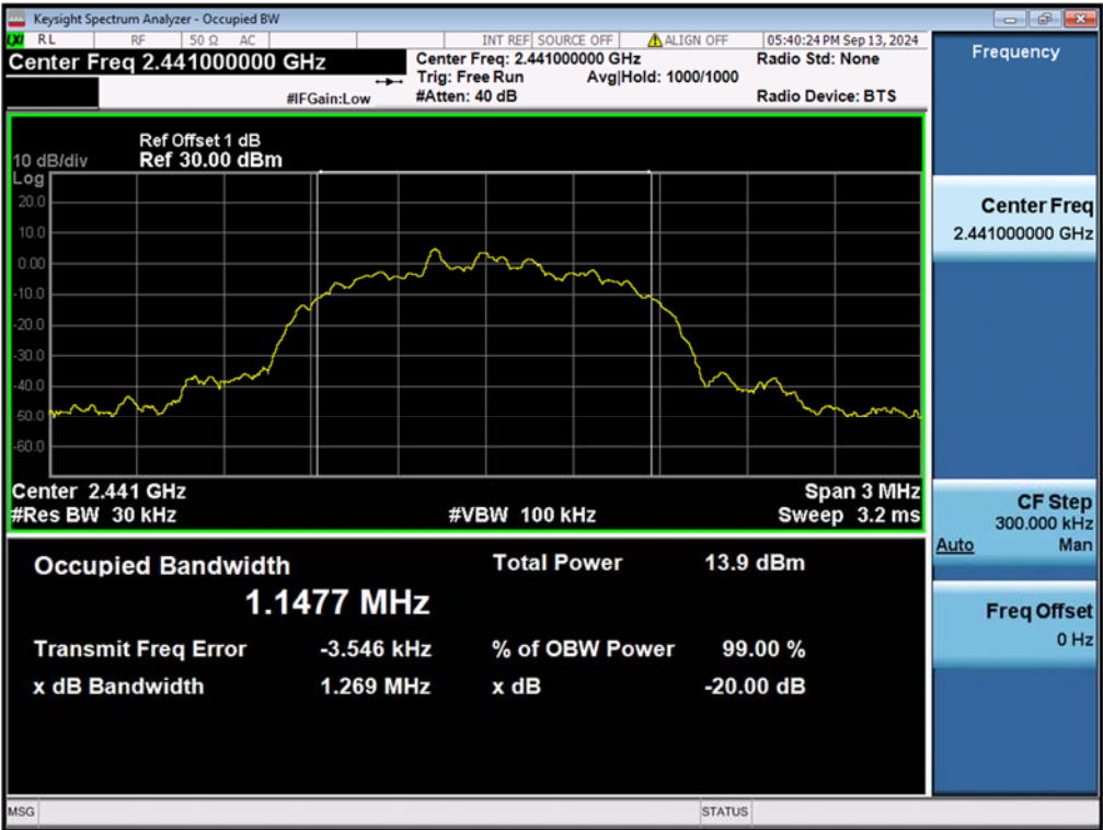
Figure 17: 20dB Bandwidth and 99% Bandwidth, 2441MHz, 8-DPSK
