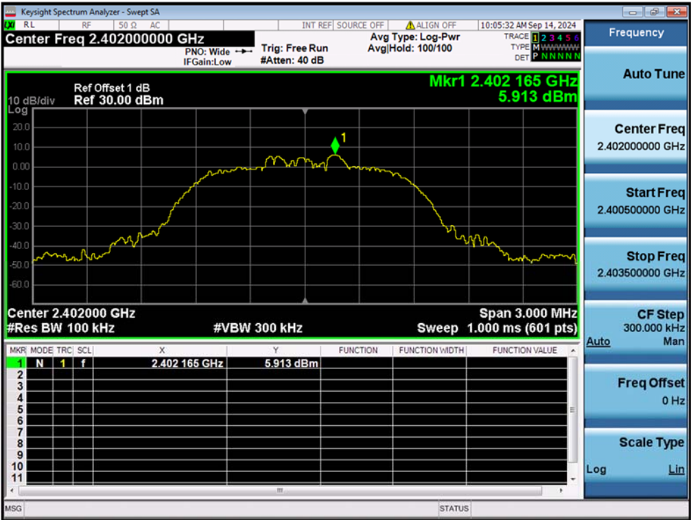
Figure 22: Conducted Spurious Emission & Authorized-band band-edge, 2402MHz, \pi/4 -DQPSK Carrier Level
