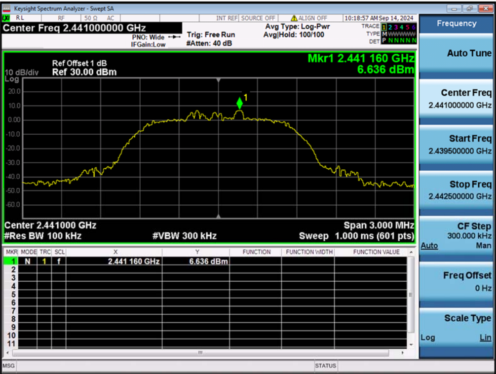
Figure 23: Conducted Spurious Emission & Authorized-band band-edge, 2441MHz, \pi/4 -DQPSK Carrier Level
