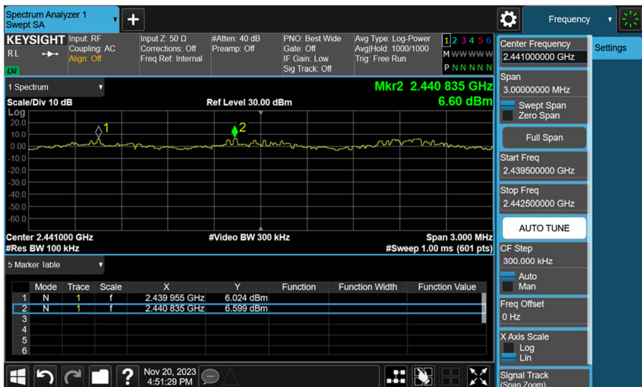
Figure 32: Hopping Frequency Separation, Hopping Mode, \pi/4 -DQPSK
