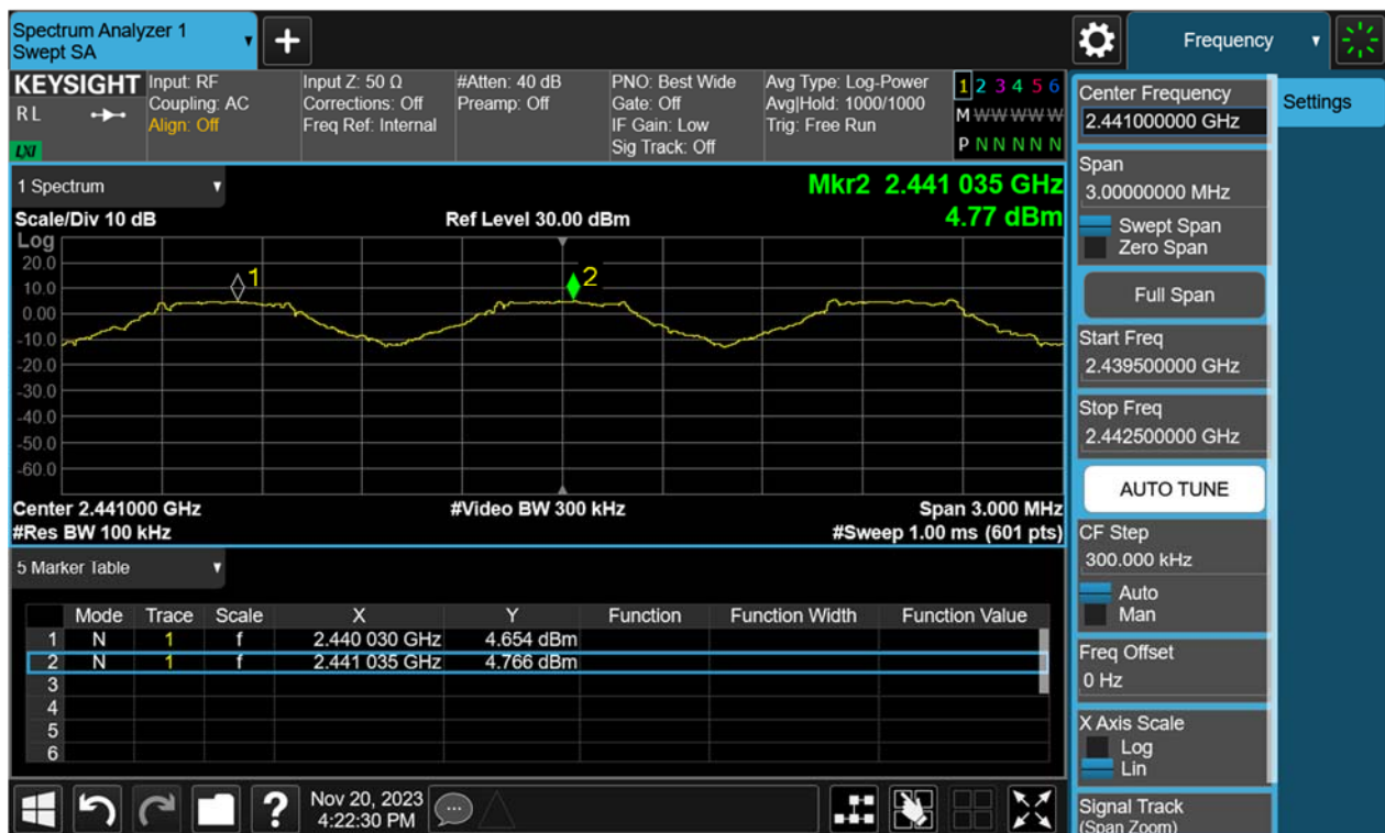
Figure 32: Hopping Frequency Separation, Hopping Mode, \pi/4 -DQPSK
