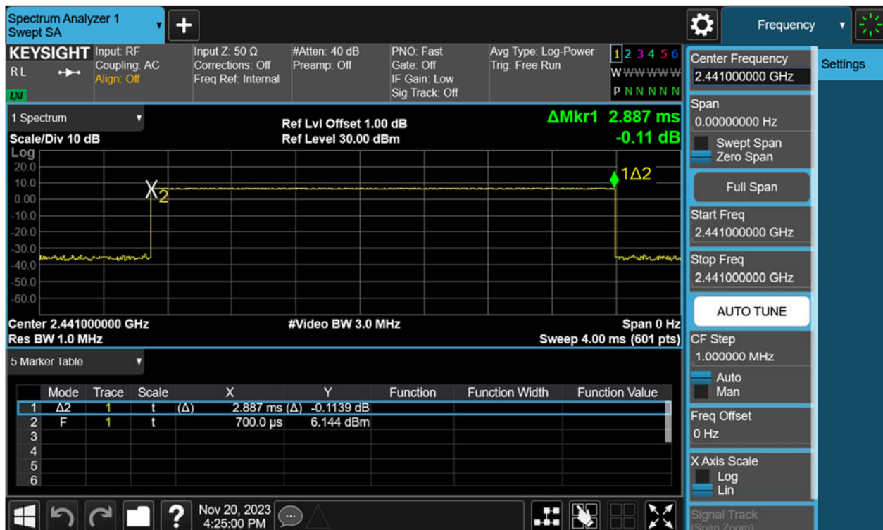
Figure 40: Time of Occupancy, 2441MHz, \pi/4 -DQPSK DH1
