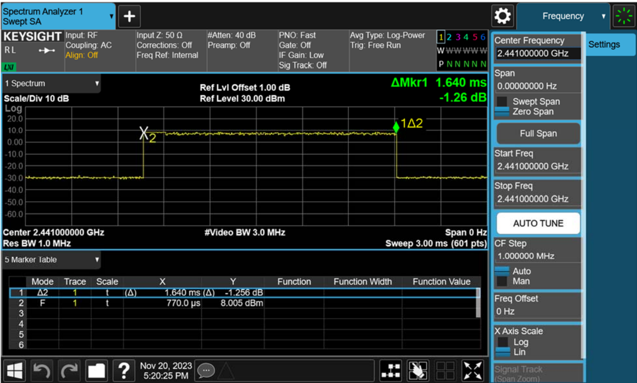
Figure 44: Time of Occupancy, 2441MHz, 8-DPSK DH3
