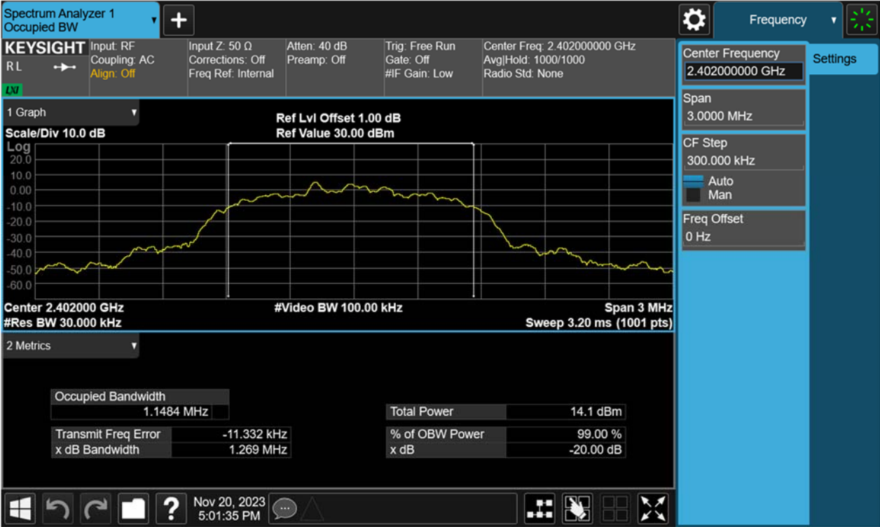
Figure 17: 20dB Bandwidth and 99% Bandwidth, 2441MHz, 8-DPSK
