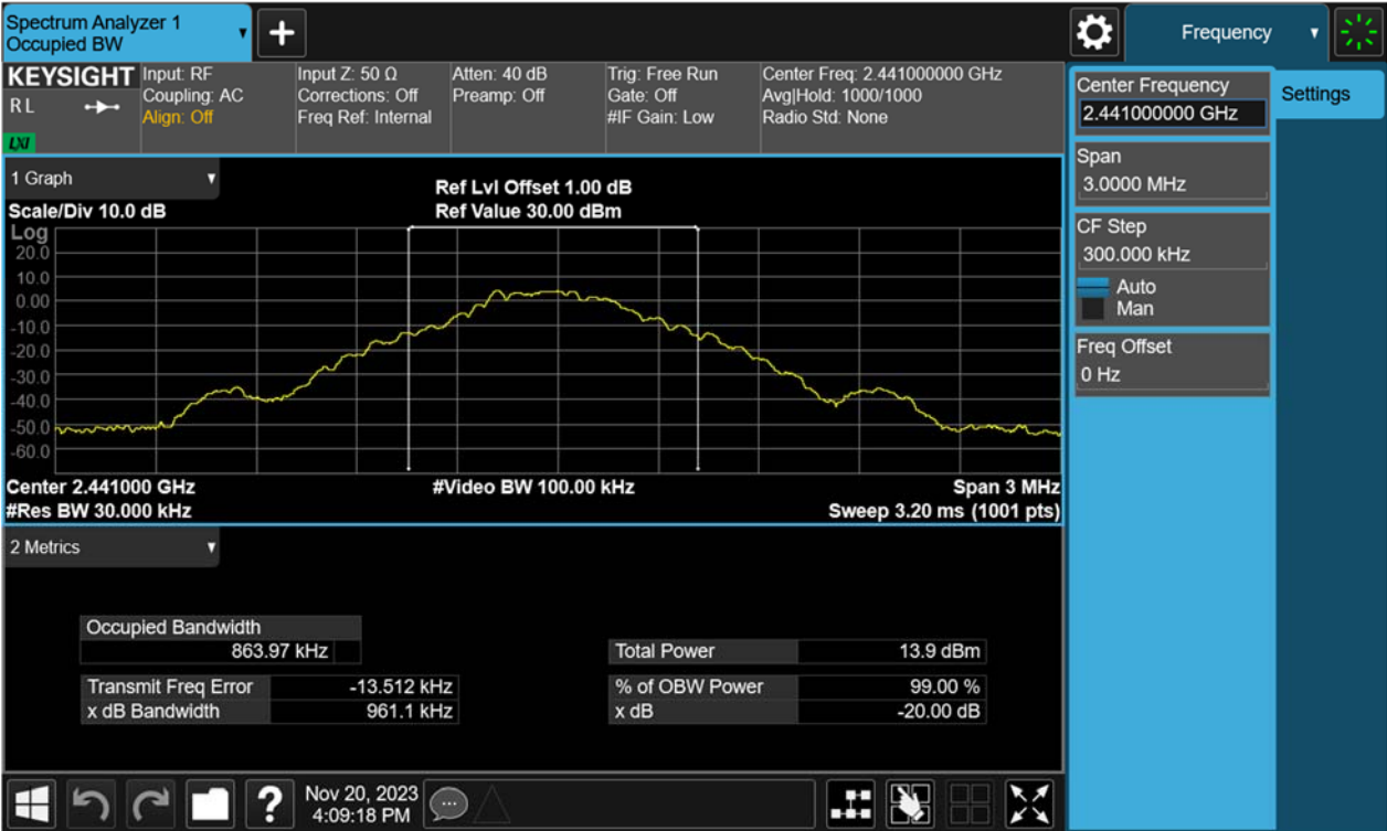
Figure 11: 20dB Bandwidth and 99% Bandwidth, 2441MHz, GFSK
