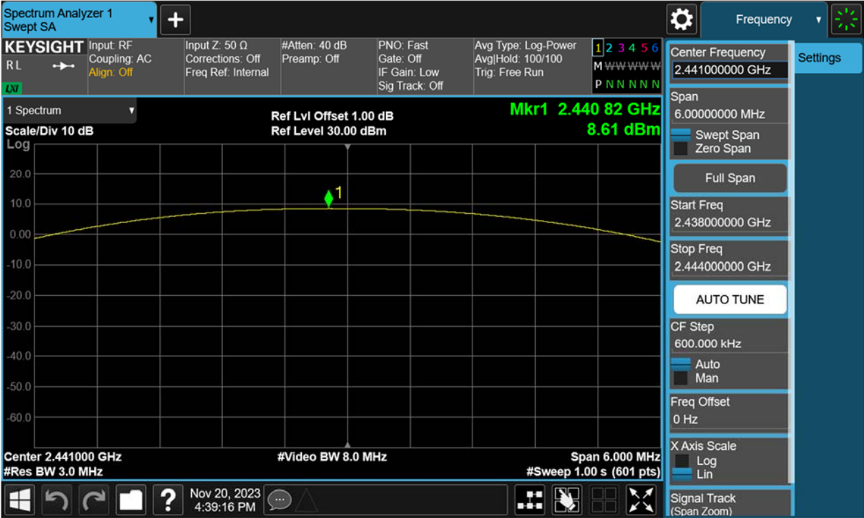
Figure 6: Maximum Peak Output Power, 2480MHz, \pi/4 -DQPSK
