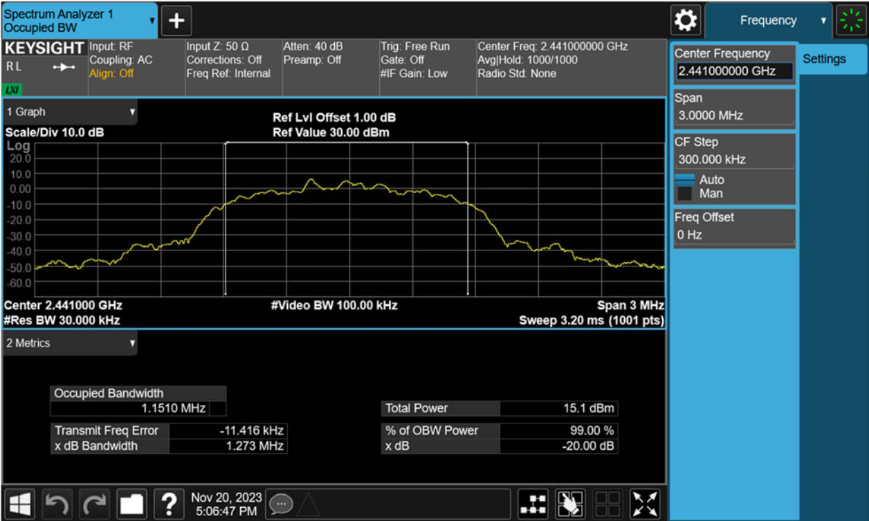
Figure 17: 20dB Bandwidth and 99% Bandwidth, 2441MHz, 8-DPSK
