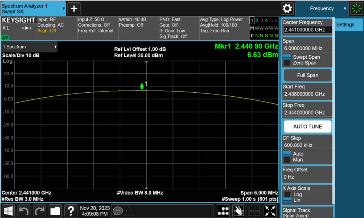
Figure 2: Maximum Peak Output Power, 2441MHz, GFSK
