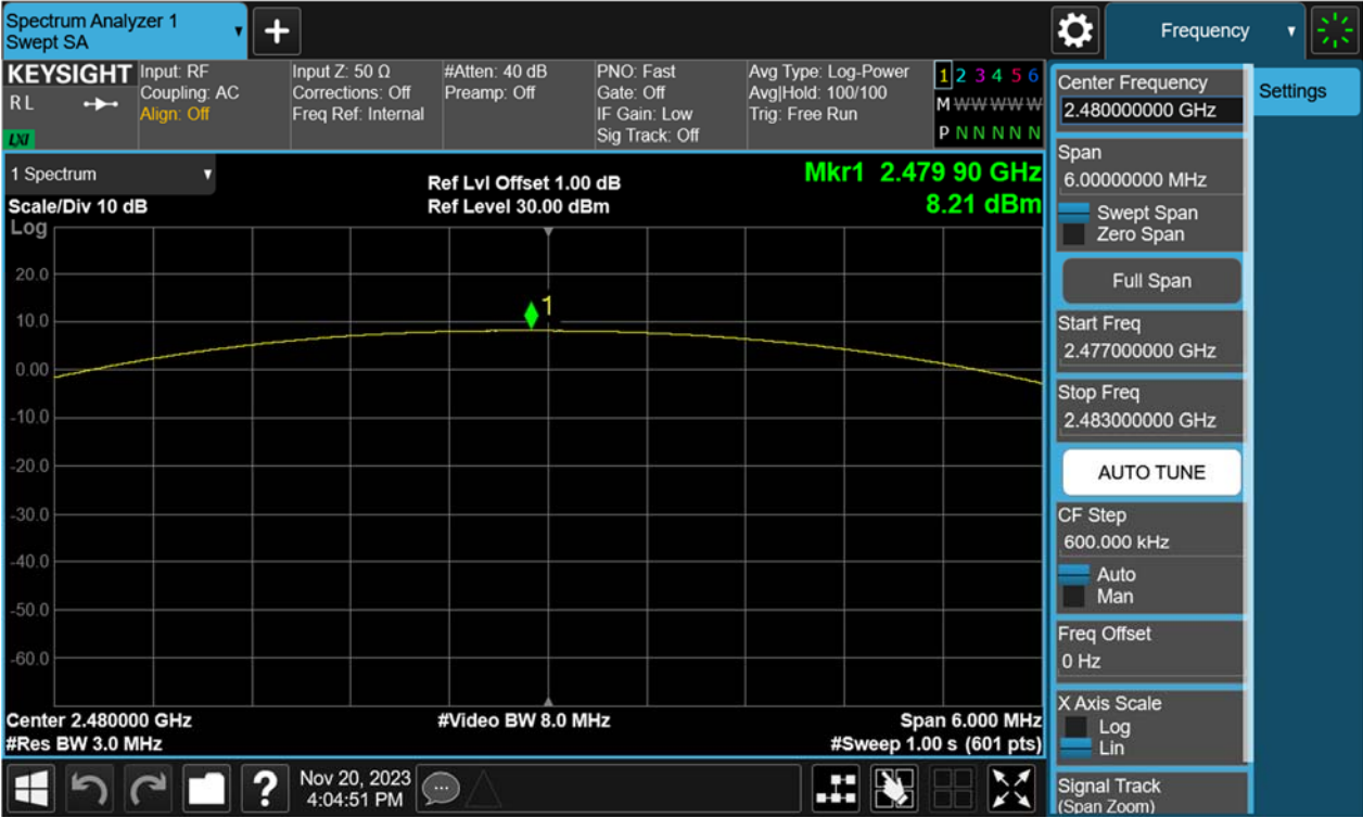
Figure 4: Maximum Peak Output Power, 2402MHz, \pi/4 -DQPSK
