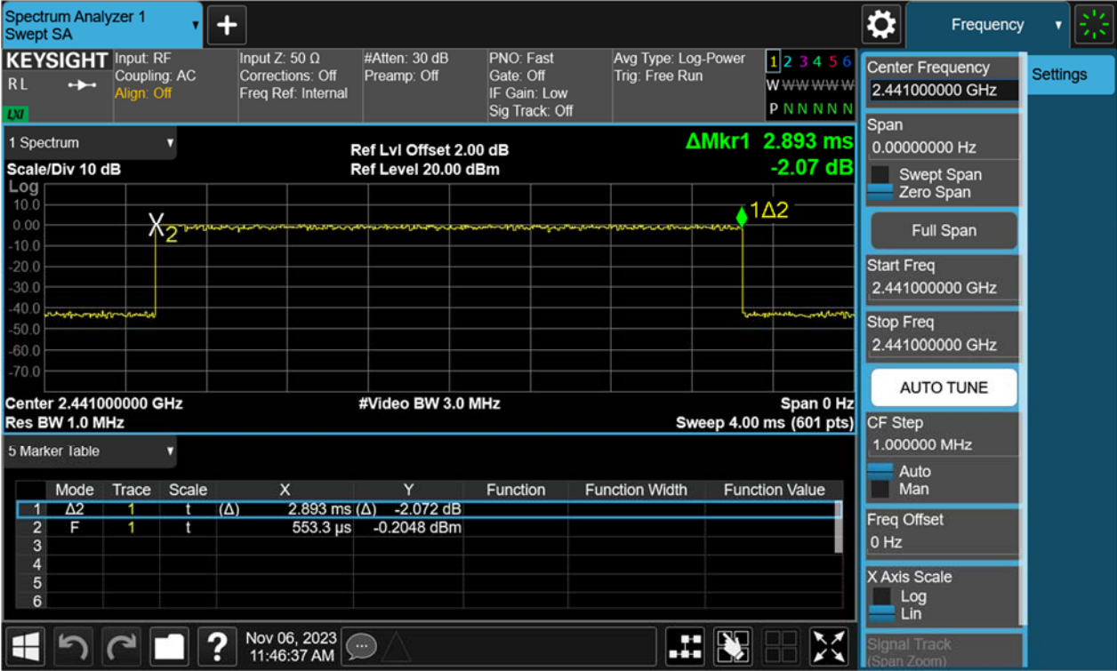
Figure 45: Time of Occupancy, 2441MHz, 8-DPSK DH5
