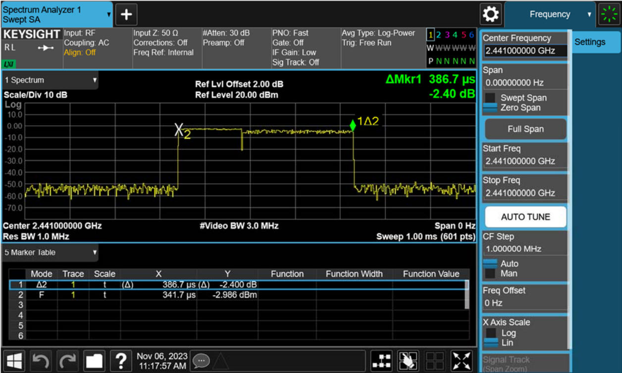
Figure 40: Time of Occupancy, 2441MHz, \pi/4 -DQPSK DH1
