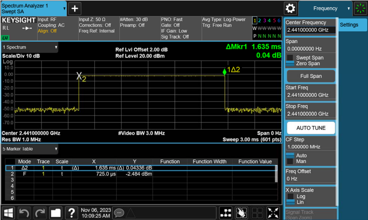
Figure 38: Time of Occupancy, 2441MHz, GFSK DH3
