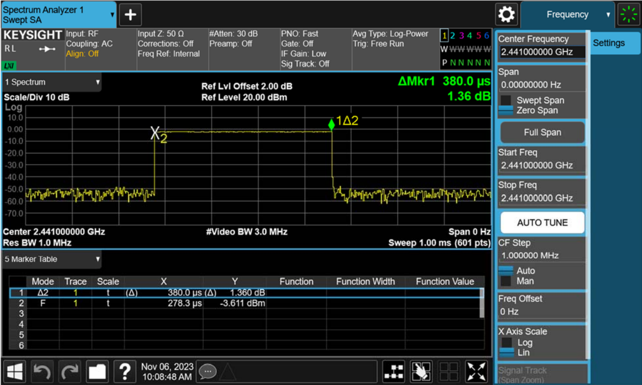
Figure 38: Time of Occupancy, 2441MHz, GFSK DH3
