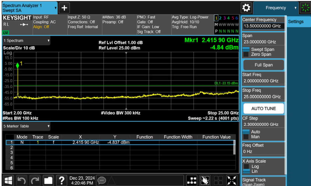
Figure 71: Conducted Spurious Emission & Authorized-band band-edge, 802.11ax(HE40), 2437MHz Carrier Level
