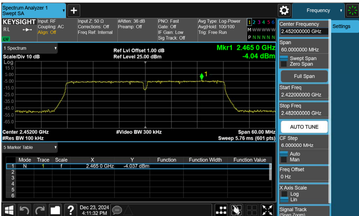
Figure 69: Conducted Spurious Emission & Authorized-band band-edge, 802.11n(HT40), 2452MHz Carrier Level
