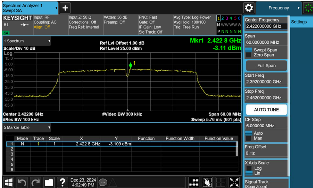
Figure 67: Conducted Spurious Emission & Authorized-band band-edge, 802.11n(HT40), 2422MHz Carrier Level
