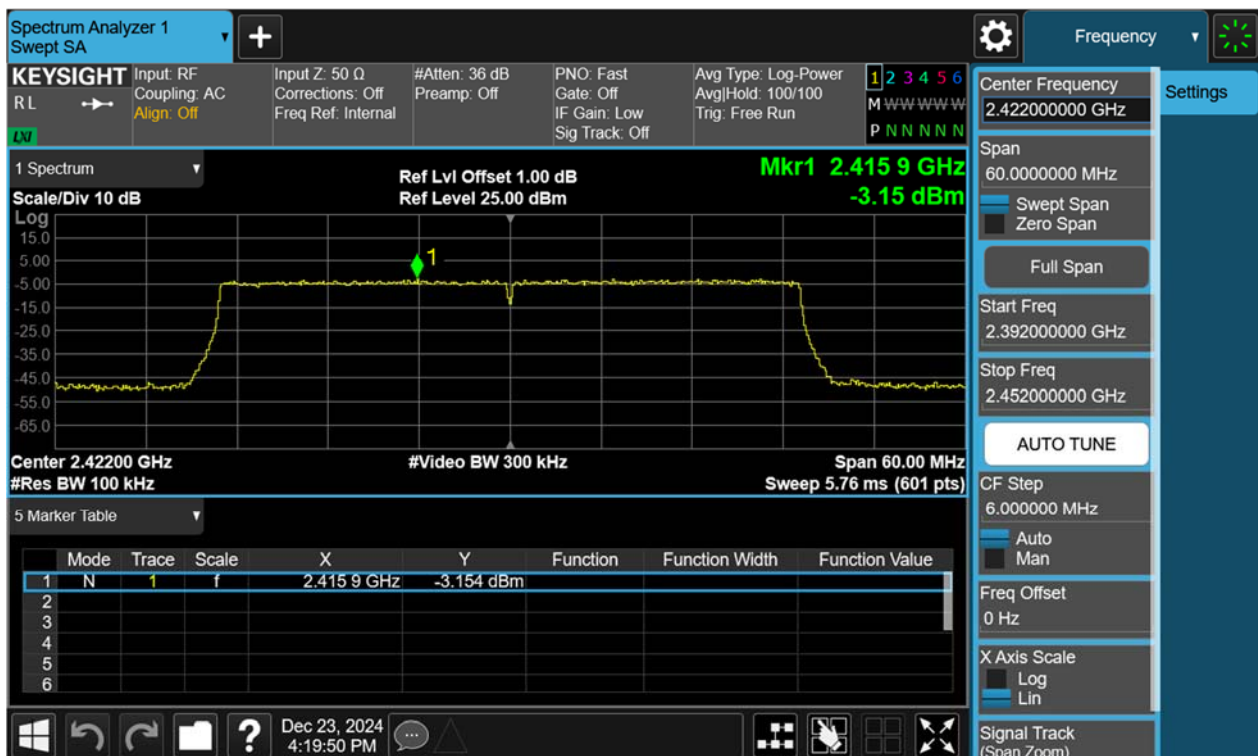
Figure 70: Conducted Spurious Emission & Authorized-band band-edge, 802.11ax(HE40), 2422MHz Carrier Level
