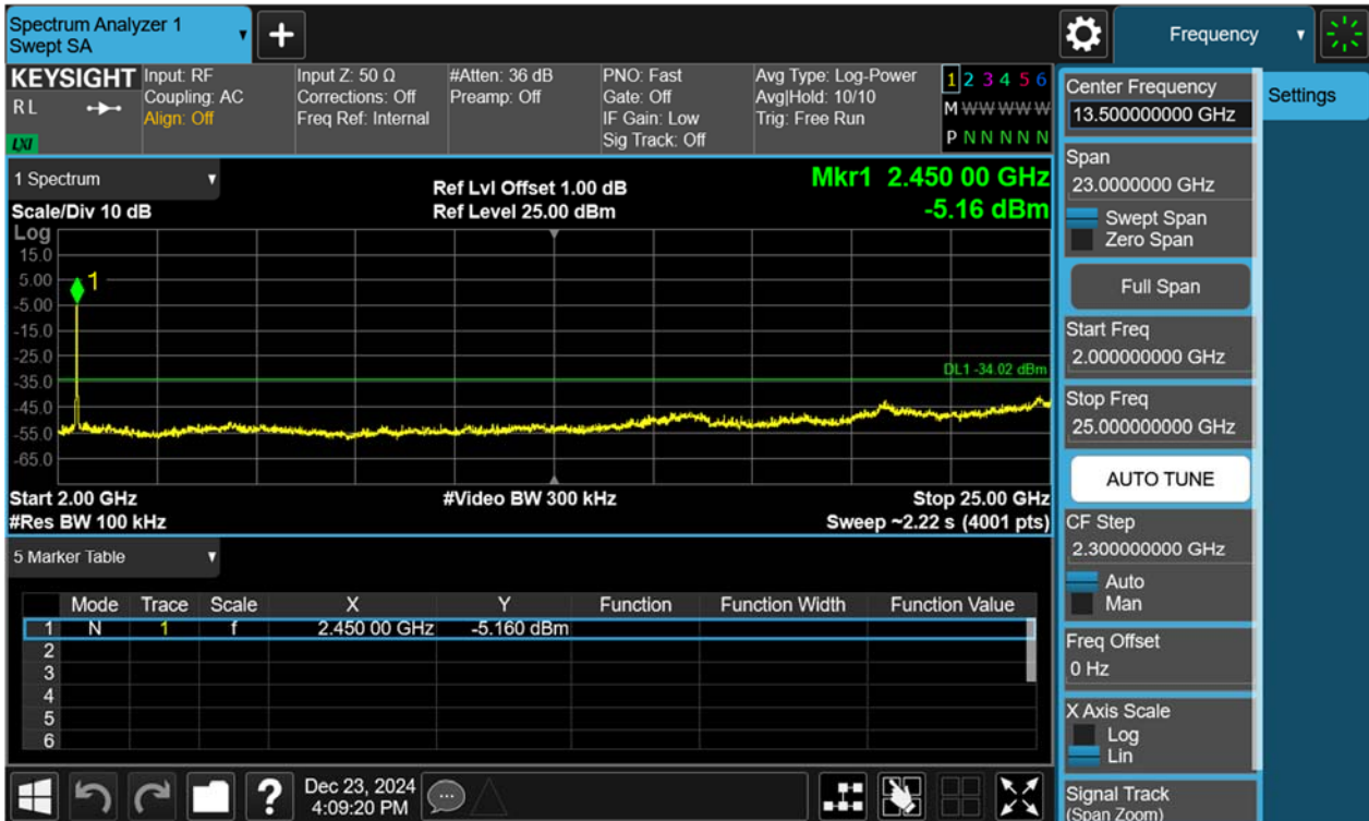
Figure 69: Conducted Spurious Emission & Authorized-band band-edge, 802.11n(HT40), 2452MHz Carrier Level
