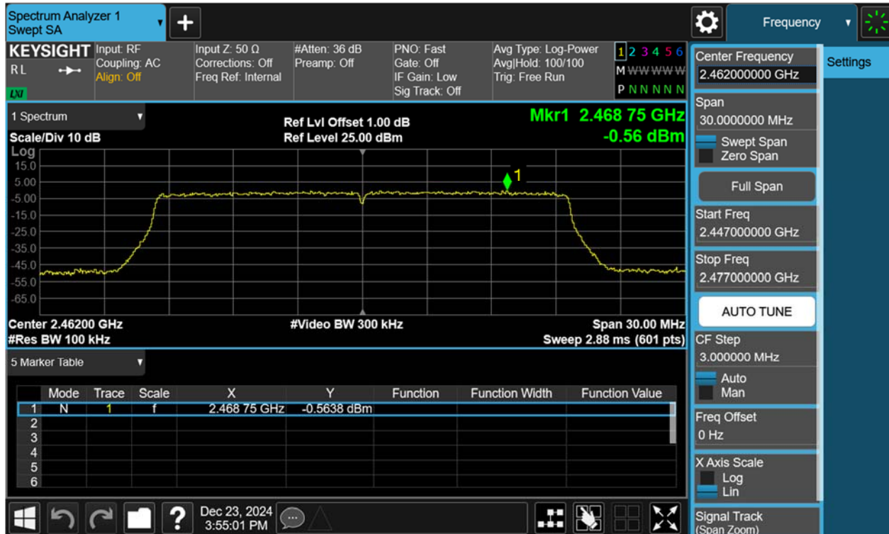
Figure 66: Conducted Spurious Emission & Authorized-band band-edge, 802.11ax(HE20), 2462MHz Carrier Level
