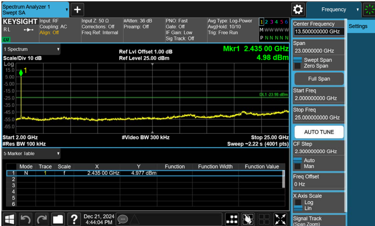
Figure 57: Conducted Spurious Emission & Authorized-band band-edge, 802.11b, 2462MHz Carrier Level
