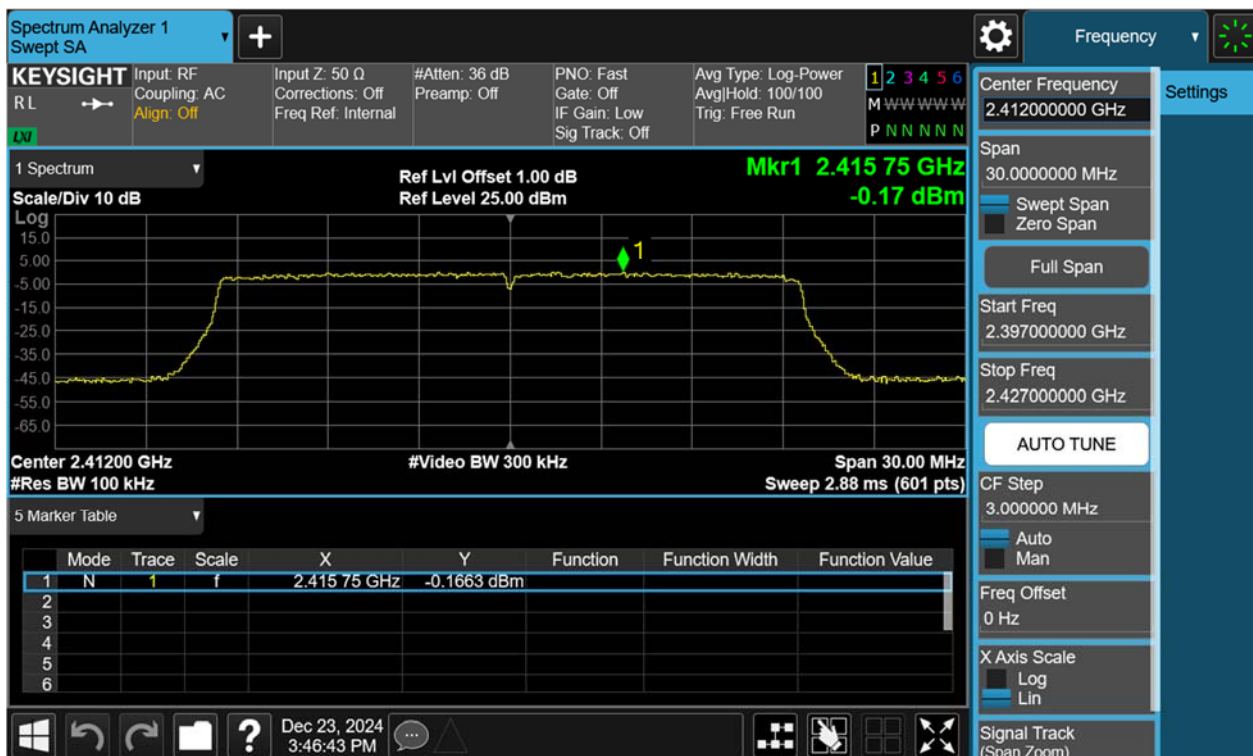
Figure 64: Conducted Spurious Emission & Authorized-band band-edge, 802.11ax(HE20), 2412MHz Carrier Level
