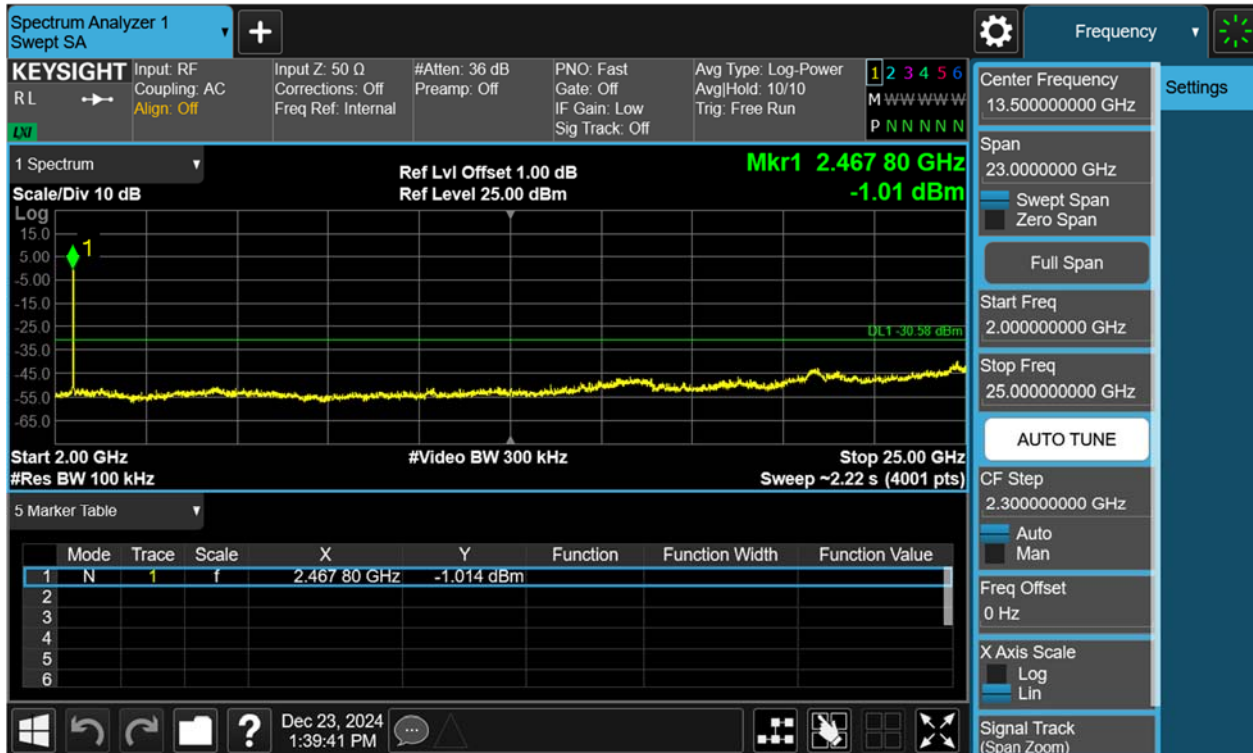
Figure 64: Conducted Spurious Emission & Authorized-band band-edge, 802.11ax(HE20), 2412MHz Carrier Level
