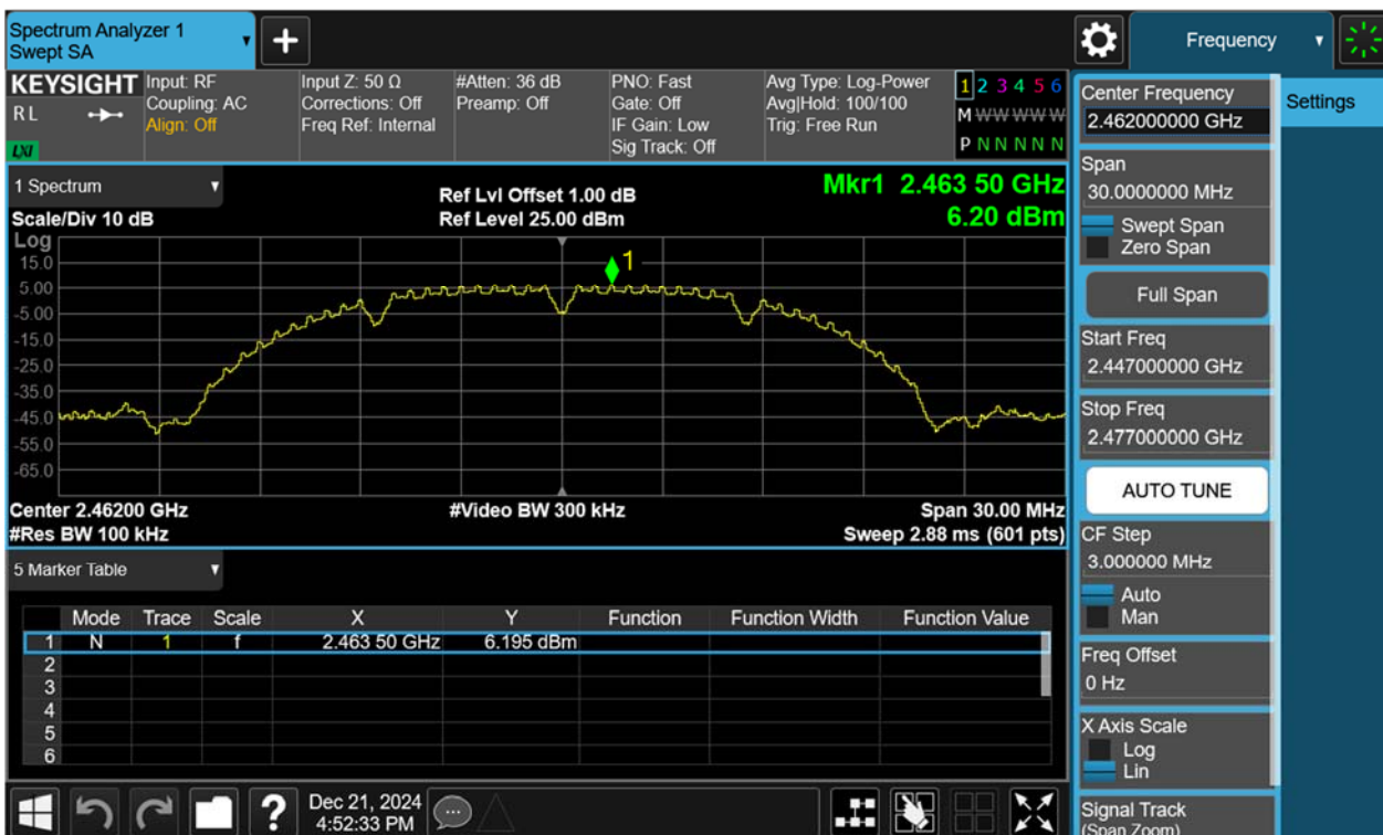
Figure 57: Conducted Spurious Emission & Authorized-band band-edge, 802.11b, 2462MHz Carrier Level
