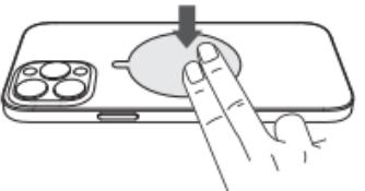
3. Paste the metal ring onto the center of the phone back by use of the alignment card
