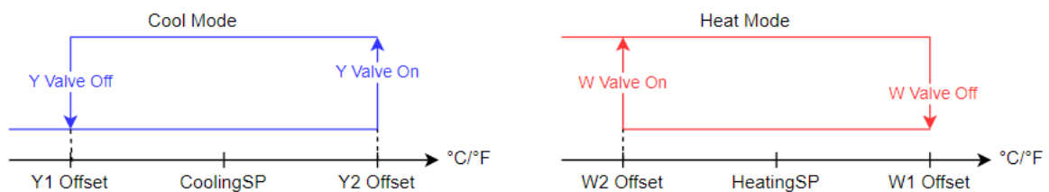
FIGURE 19: TWO PIPE COOLING AND HEATING MODE
