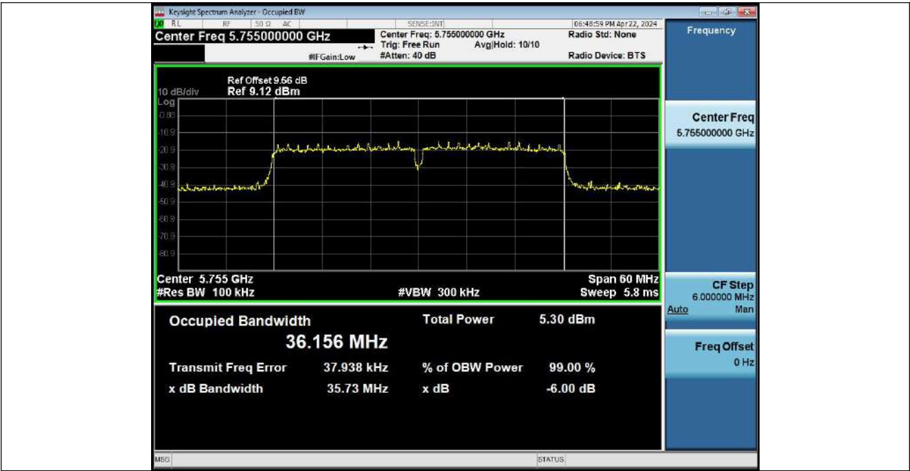
-6dB Emission Bandwidth NVNT ANT1 802 11n(HT40) 5795 40M
