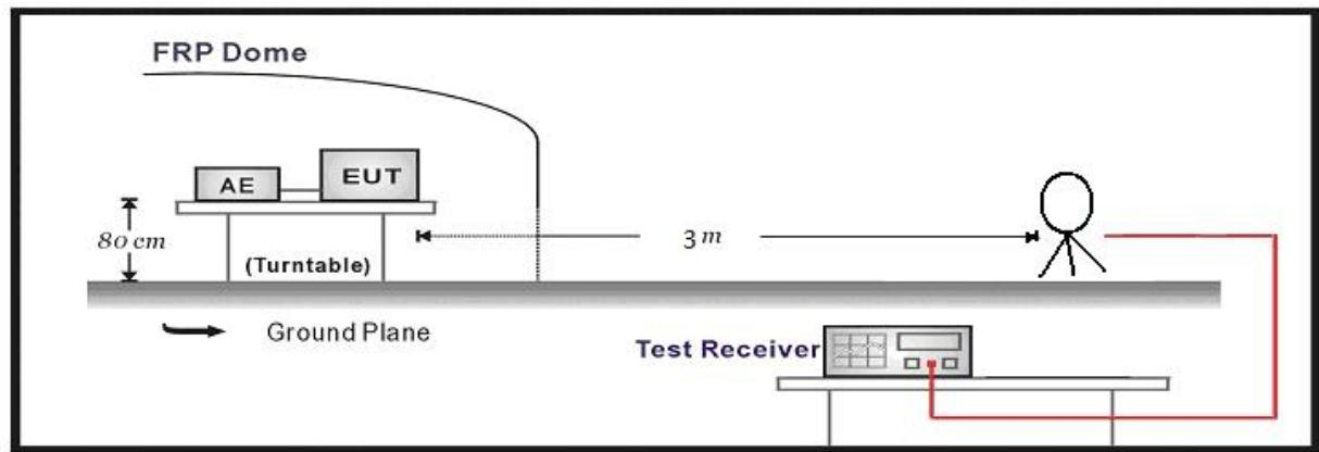
Below 1GHz Test Setup:
