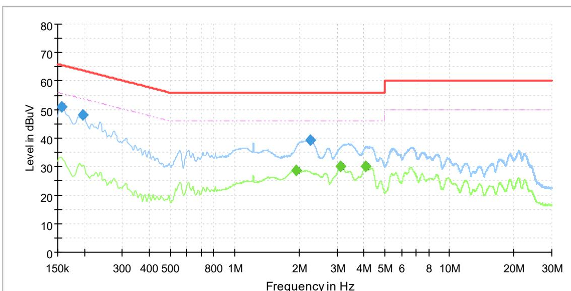
During the test, the Conducted Emission from 150kHz to 30MHz was performed in all modes with all channels, and all antennas. Bluetooth(LE\_2M), Channel 0, Antenna 1 are selected as the worst condition. The test data of the worst-case condition was recorded in this report.
