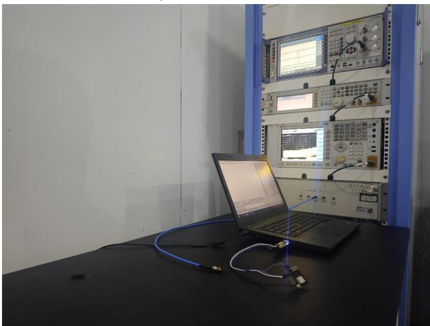
**Radiated Spurious Emissions Below 1GHz**
