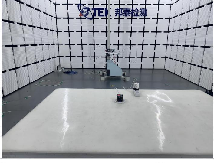
A photograph of an anechoic chamber, similar to the one above. The floor is white and reflective. In the center, there is a small black device on a white circular platform. A tripod-mounted antenna is positioned above the device. The walls of the chamber are covered in white absorptive panels with a grid pattern. The BTEK logo and text '邦泰检测' are visible on the wall. |
