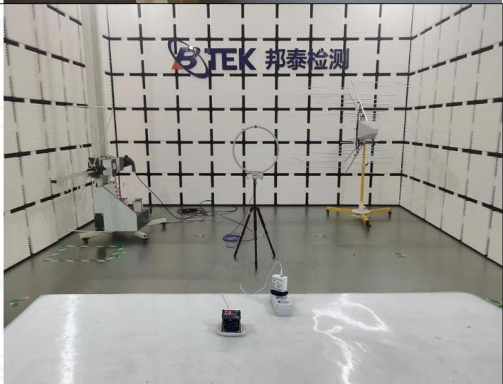
A photograph of an anechoic chamber. The floor is white and reflective. In the center, there is a small black device on a white circular platform. A tripod-mounted antenna is positioned above the device. The walls of the chamber are covered in white absorptive panels with a grid pattern. The BTEK logo and text '邦泰检测' are visible on the wall.                            |
