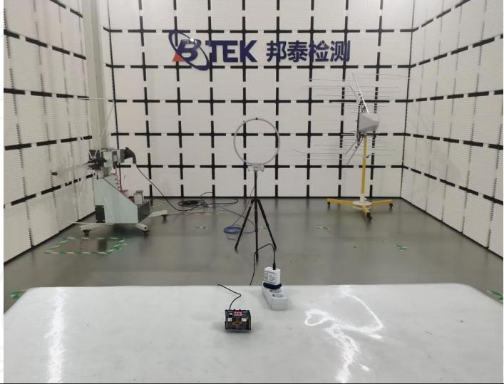
A photograph of an anechoic chamber. The floor and walls are covered with a grid of metal panels. In the center, there is a white rectangular table with a small electronic device on it. A tripod-mounted antenna is positioned above the device. The BTEK logo is visible on the wall.  |
