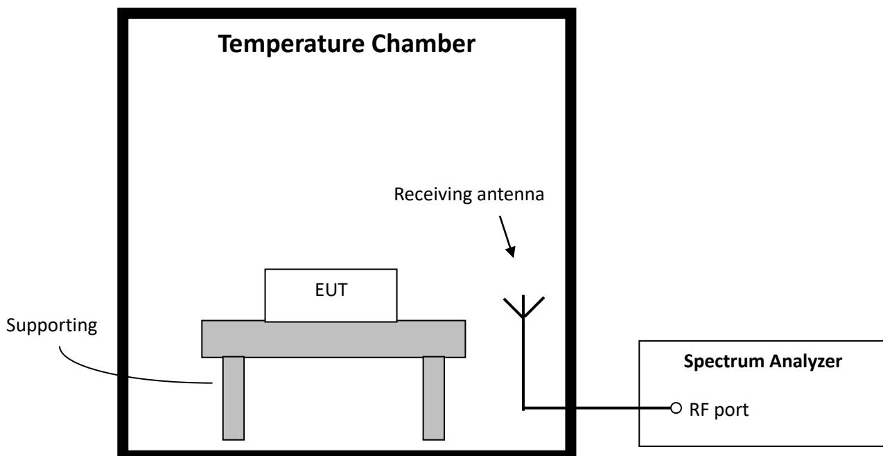
**TEST REPORT****5.3 Test procedure and test setup**
