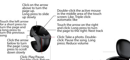
The left and right page turning of the Anzuo system is not sensitive. Please switch to a compatible system. Press and hold the left and right buttons simultaneously (for 3 seconds) until the blue light comes on, successfully switching to compatible systems.
