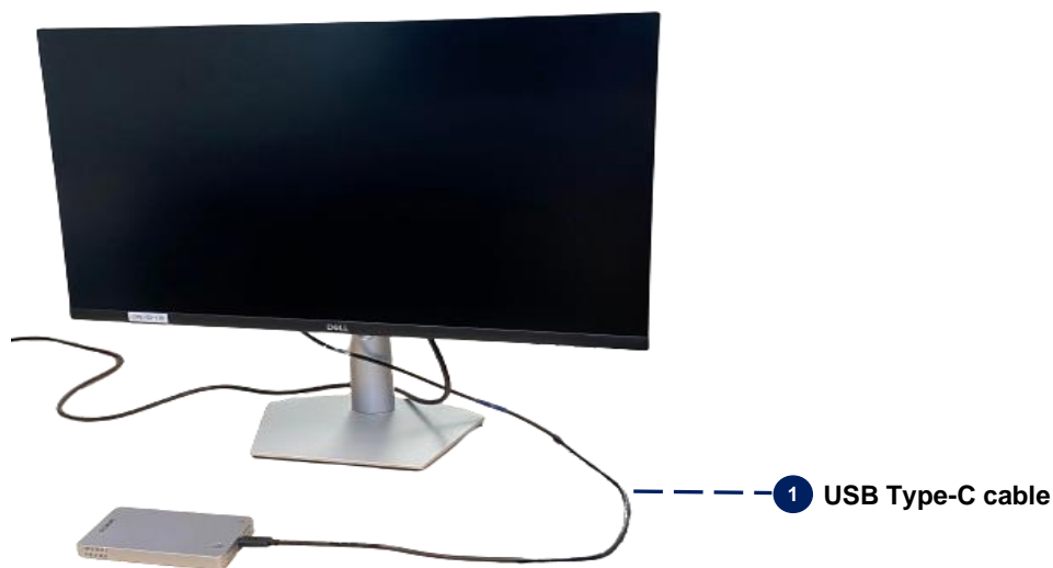
Figure 3: Connecting to your monitor without USB Type-C hub
