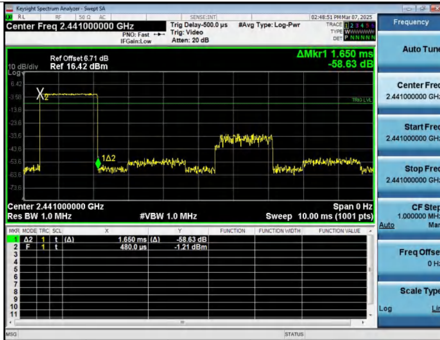
Dwell Time (Hopping) NVNT_ANT1_2-DH3_2441_00_Accumulated
