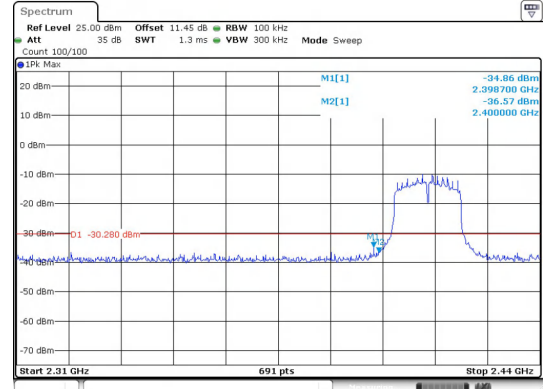
Out Of Band Emission IEEE 802.11g_Channel 1_20MHz_Antenna 0
