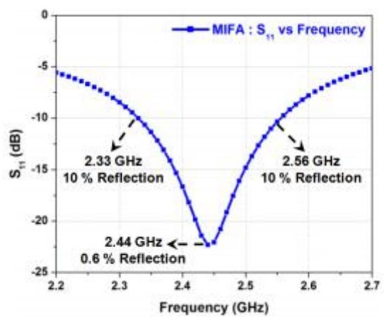
Antenna measurements such as VSWR were measured with an Agilent E5071C vector network analyzer. Radiation patterns were measured with a CMT Planar 804/1 vector network analyzer in a Howland and Company 3100 chamber equivalent. Phase center is nine inches above the Phi positioner.
