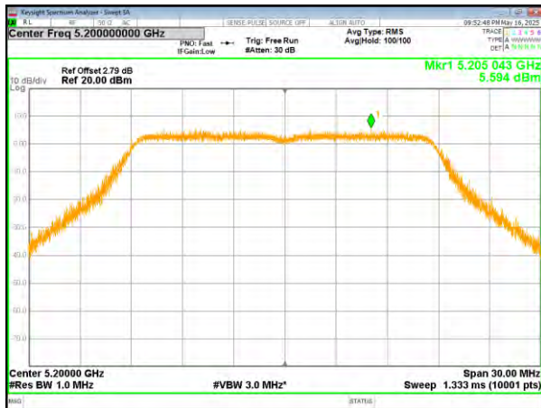
(802.11ac20) PSD plot on channel 48
