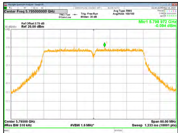
(802.11n40) PSD plot on channel 159
