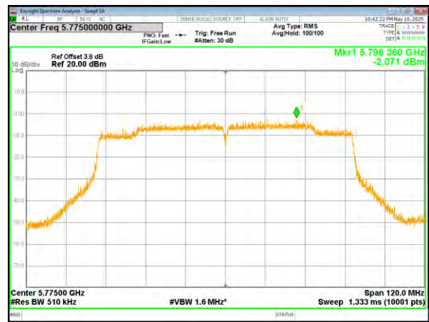
(802.11ac80) PSD plot on channel 155
