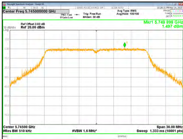
(802.11ac20) PSD plot on channel 157
