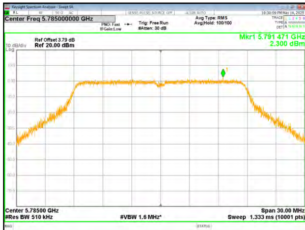
(802.11ac20) PSD plot on channel 165
