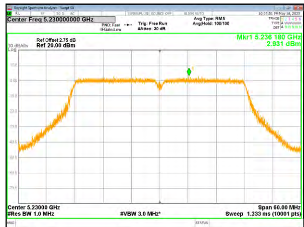
(802.11n40) PSD plot on channel 46
