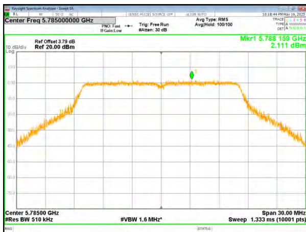
(802.11a) PSD plot on channel 157
