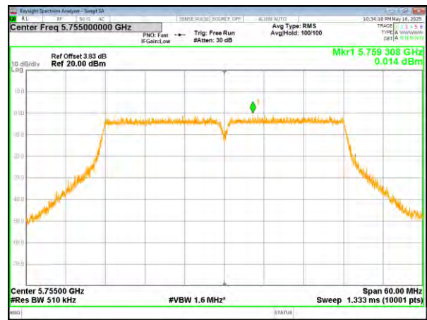
(802.11n40) PSD plot on channel 159
