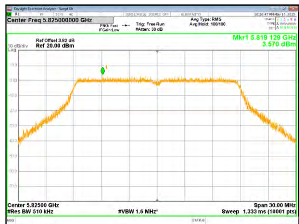
(802.11n20) PSD plot on channel 165
