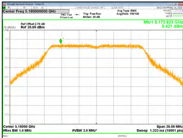
(802.11a) PSD plot on channel 36
