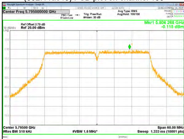
(802.11ac40) PSD plot on channel 159
