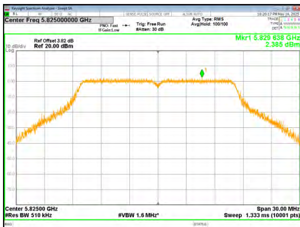
(802.11a) PSD plot on channel 165
