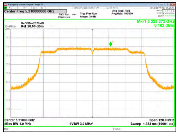
(802.11ac80) PSD plot on channel 42
