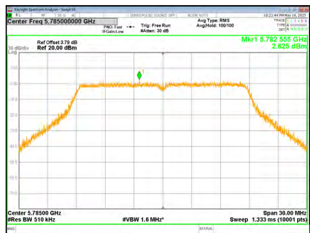
(802.11n20) PSD plot on channel 157
