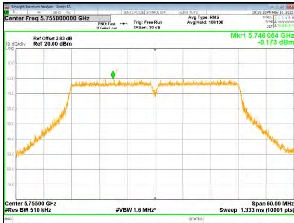
(802.11ac40) PSD plot on channel 159
