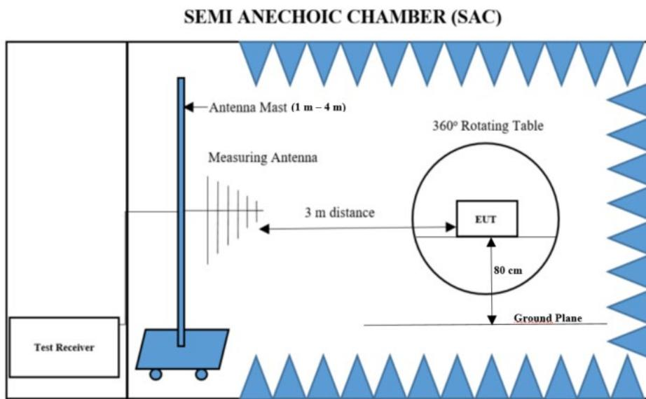
Radiated measurements from 9 kHz – 30 MHz and 30MHz – 1 were performed using an active loop antenna and Linear polarized Logarithmic Periodic Broadband Antenna, respectively with a measuring distance of 3 m inside SAC as shown in the above test setup diagrams.
