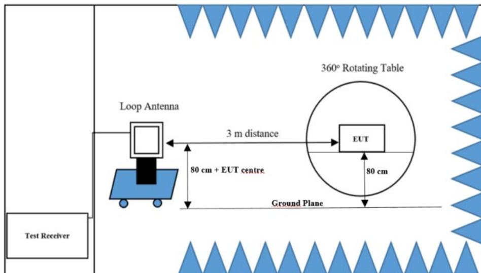
Radiated measurements setup (30 MHz – 1 GHz)
