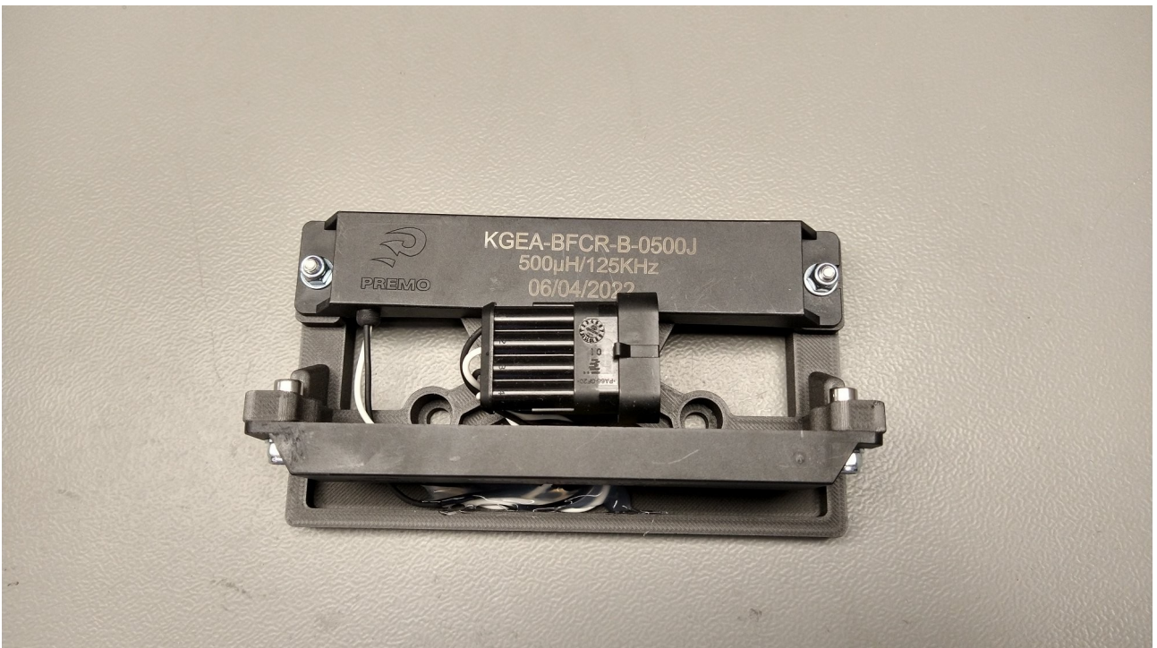
Abbildung 4: Near-field transmitting antennas (top view)
