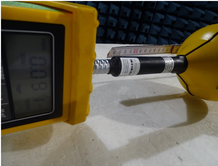
Photograph 2 : Measurement H-Field, worst case position, distance 20.0 cm
