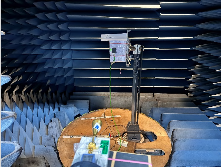
Photograph 7: EUT test setup in the anechoic chamber (mixer set-up)
