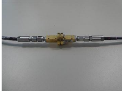
Figure 4: Back-to-Back Setup of two 08K620-385 waveguide adaptors.
