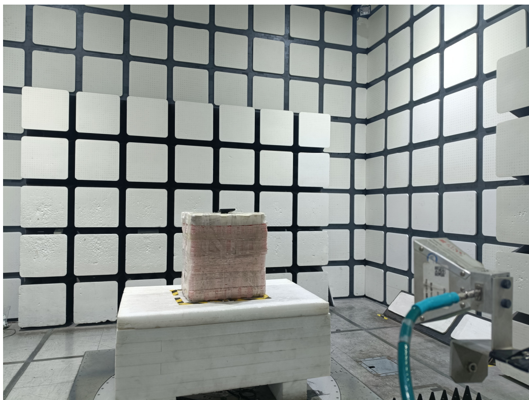
Radiated Emissions View (18-25 GHz)
