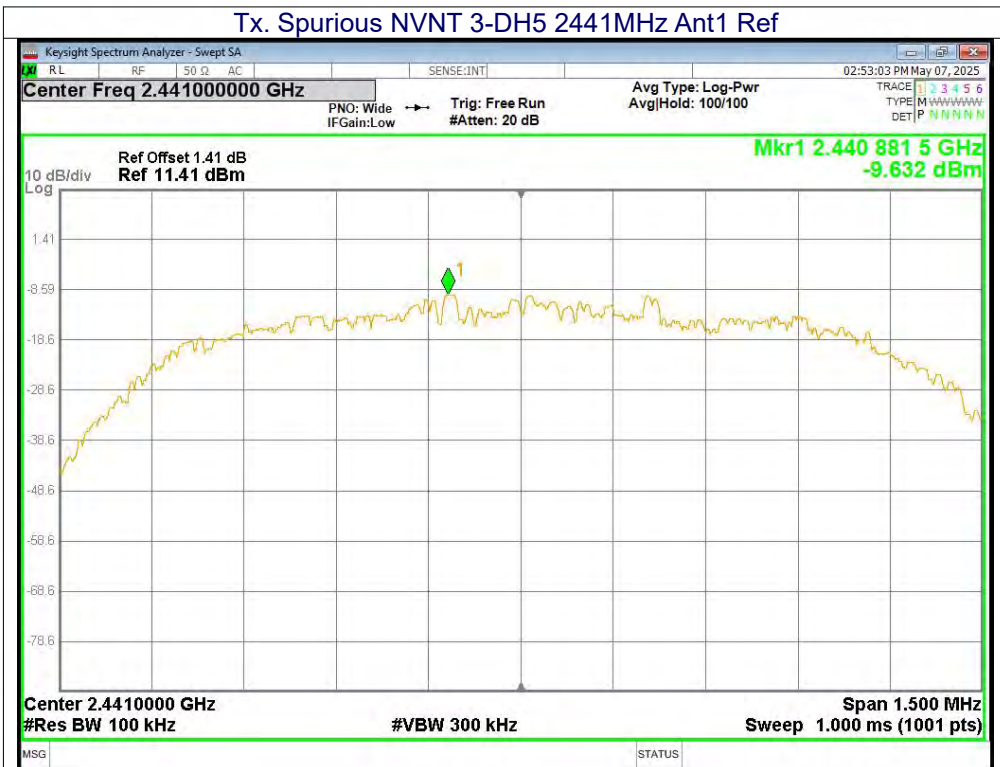
Tx. Spurious NVNT 3-DH5 2441MHz Ant1 Emission
