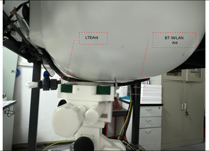
Positioning relative to the head phantom (Separation distance of 0mm)
