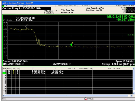
Out Of Band Emission(Right) 8DPSK_3-DH5_Channel Hopping
