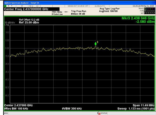
In-Band Reference Level IEEE 802.11b_Channel 6_20MHz_Antenna 0
