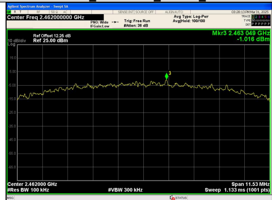
In-Band Reference Level IEEE 802.11b_Channel 11_20MHz_Antenna 0
