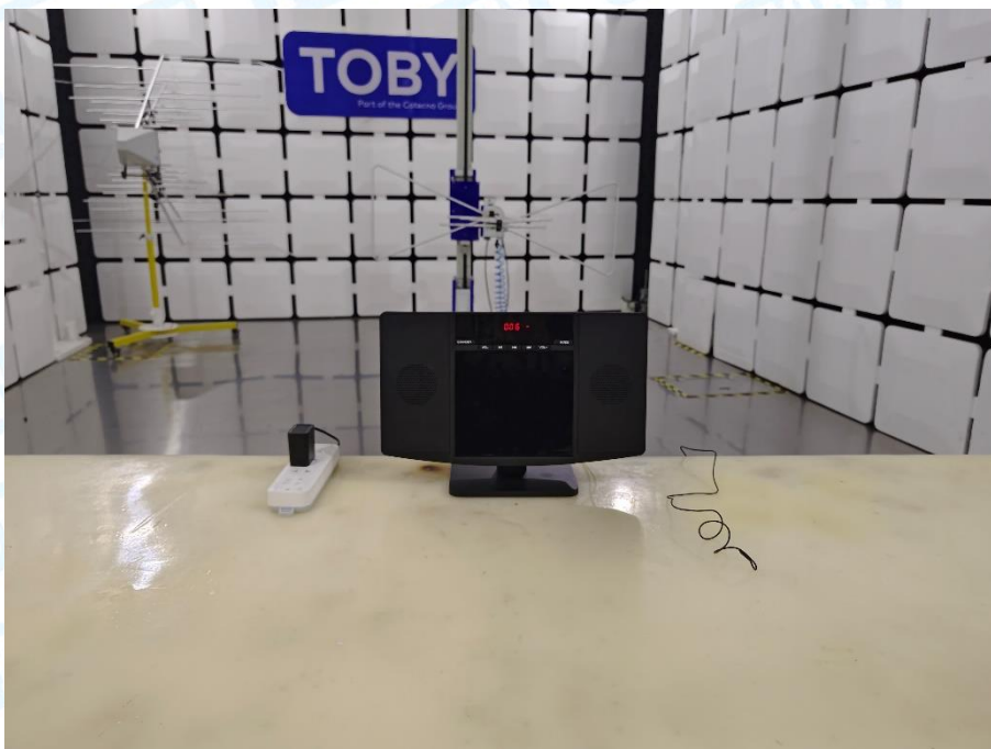
Photo of Setup for Radiated Emission (30MHz~1GHz)
