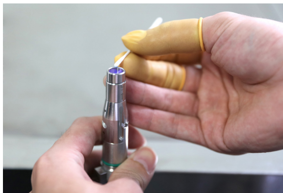
7-3 Cleaning protective lens with swabs
