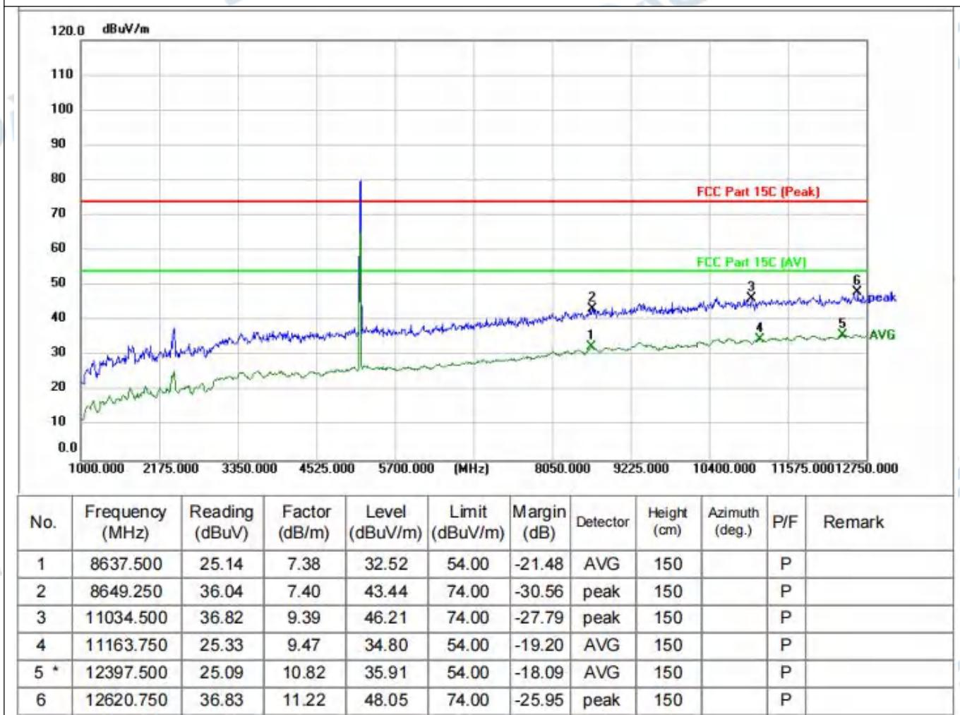
TM1 / Polarization: Vertical / Band: 5150-5250 MHz / BW: 20 / CH: L
