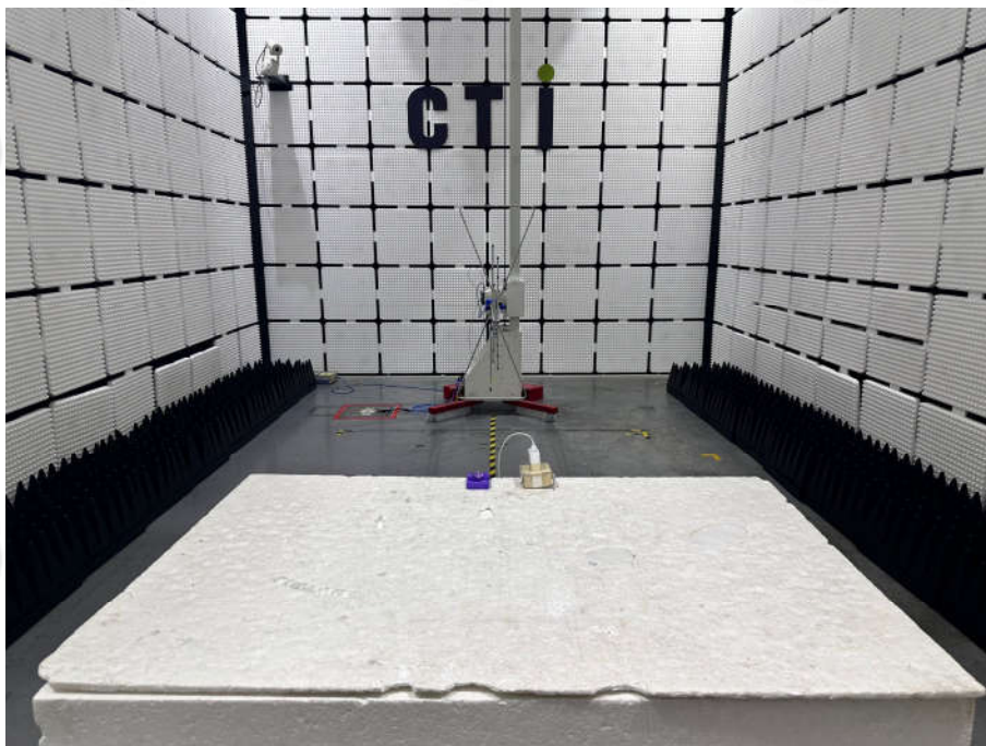
Radiated Emissions Test Setup (30MHz-1GHz)Mode a
