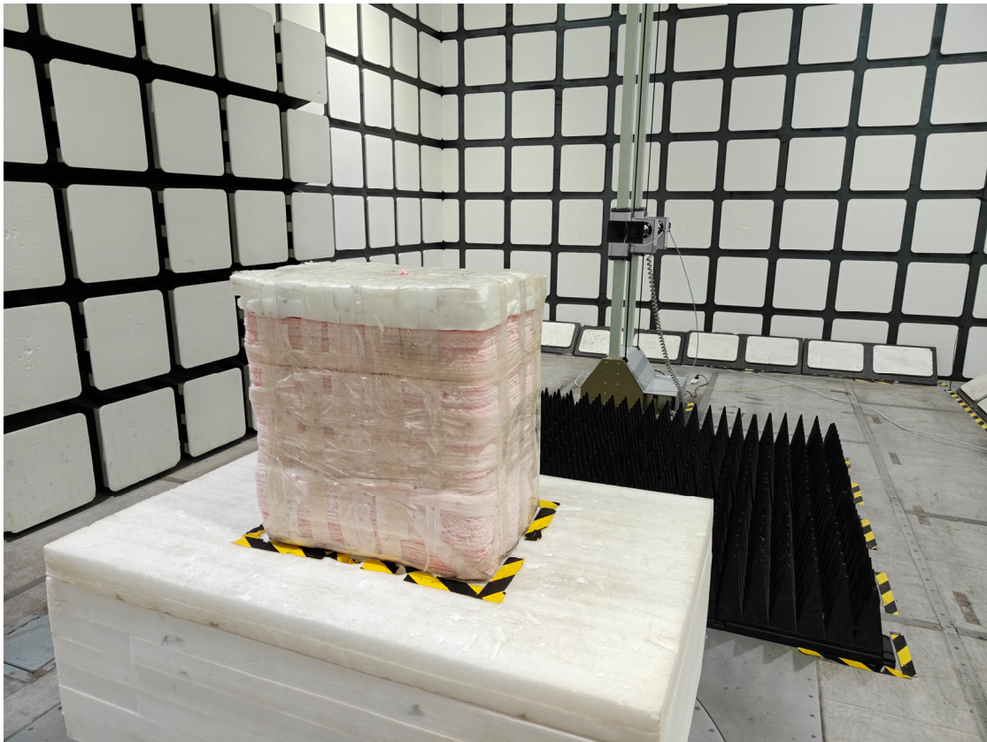
Radiated Emissions View (18-25 GHz)
