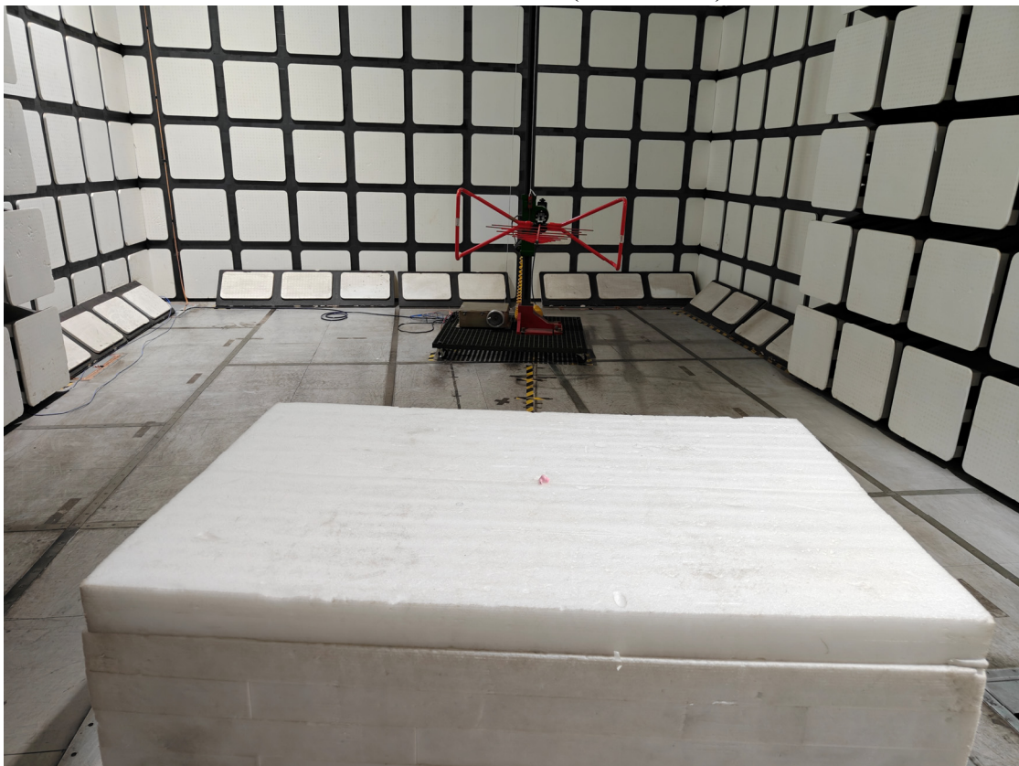
Radiated Emissions View (Below 1 GHz)
