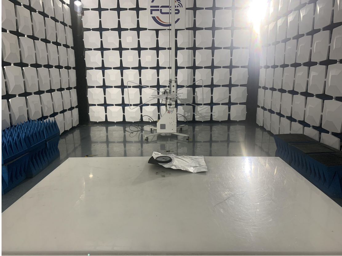
Above 1GHz for radiated emission test setup
