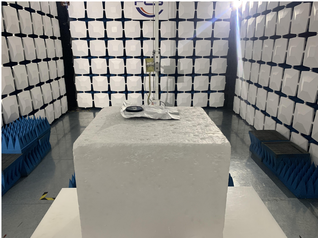
Above 1GHz for radiated emission test setup
