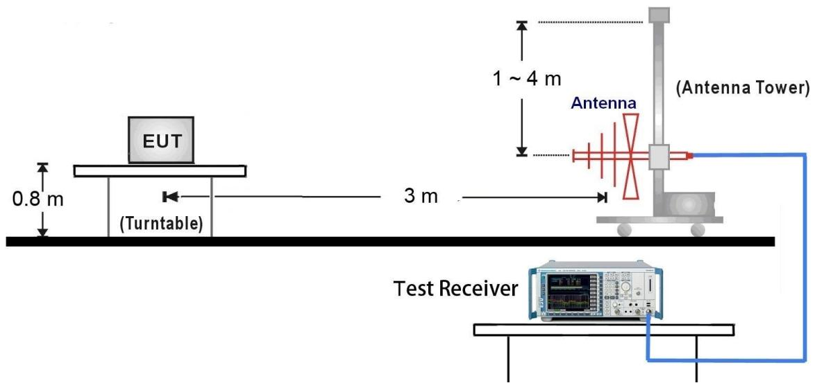
1GHz ~ 18GHz Test Setup:
