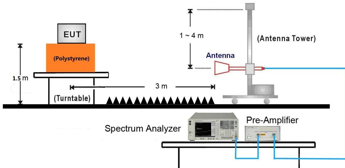
18GHz ~25GHz Test Setup:
