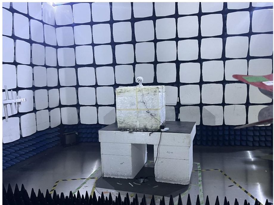
Radiation Emission Test Setup (1GHz to 18GHz)
