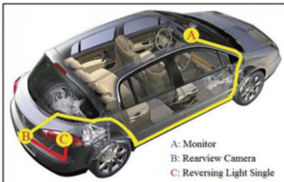
**4.1** As shown in the figure, the yellow line is a schematic wiring diagram of the extension line of the rearview camera. (From A to B)
