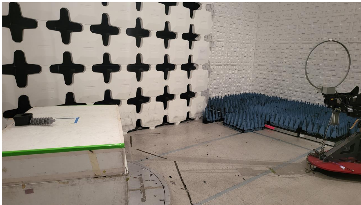
Figure 2. Radiated Emissions Test Setup, .15 MHz to 30 MHz
