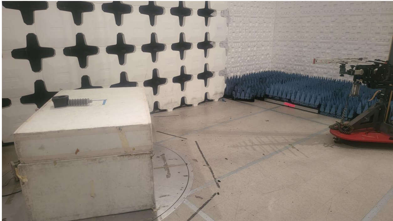
Figure 4. Radiated Emissions Test Setup, 200 MHz to 1GHz
