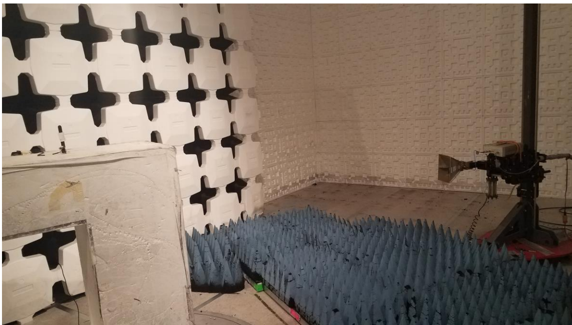
Figure 4. Radiated Emission Test Setup, above 1 GHz
