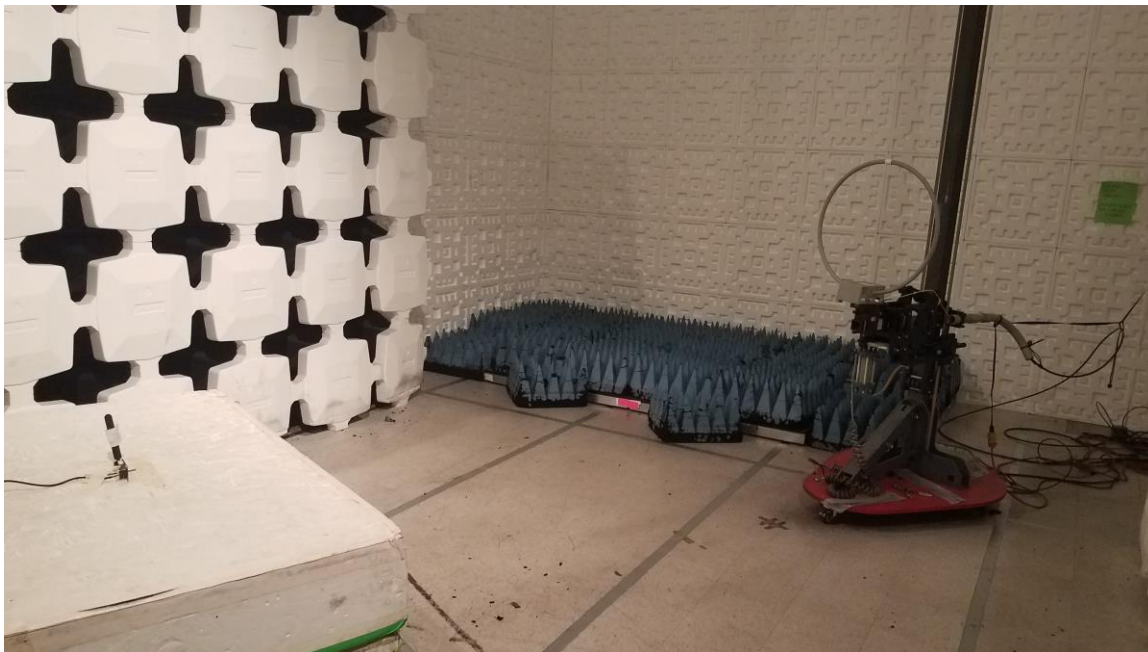
Figure 2. Radiated Emissions Test Setup, .15 MHz to 30 MHz
