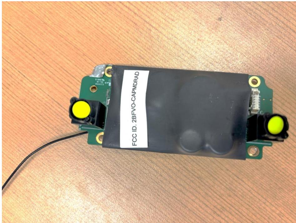
The radio module is encased in a protective layer of heat shrink to ensure durability during installation in host products. The FCC ID will be affixed to the module as illustrated in the image above and will remain visible throughout the installation process.
