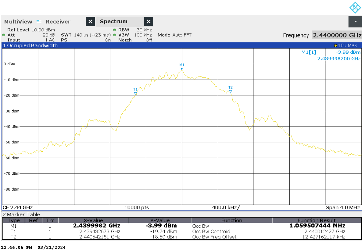
Figure 33 99% Occupied Bandwidth. 1MHz channel bandwidth, channel 2440MHz
