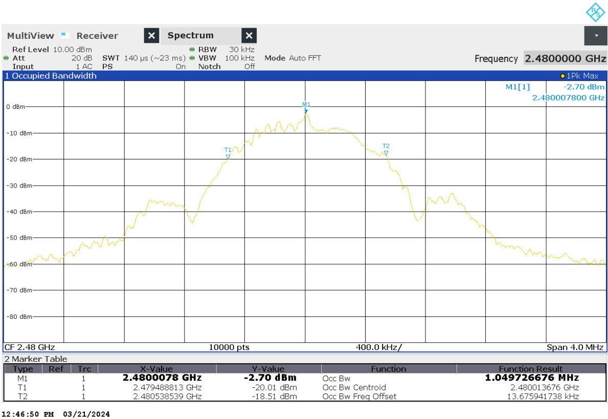
Figure 34 99% Occupied Bandwidth. 1MHz channel bandwidth, channel 2480MHz
