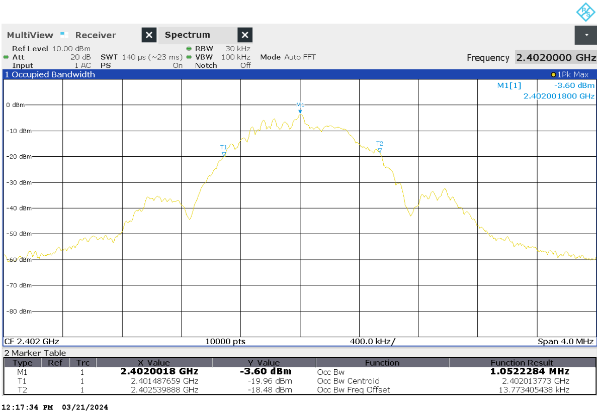
Figure 32 99% Occupied Bandwidth. 1MHz channel bandwidth, channel 2402MHz
