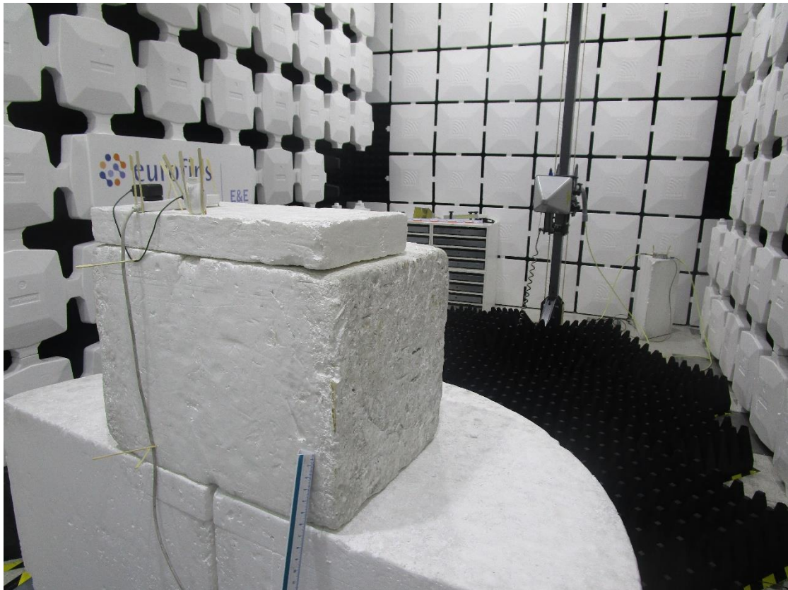
Radiated emissions tests 1-18GHz
