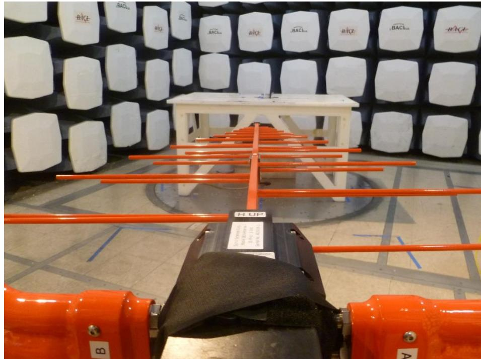
**1.6 Radiated Spurious Emissions: 30MHz - 1GHz Rear View at 3 meters**
