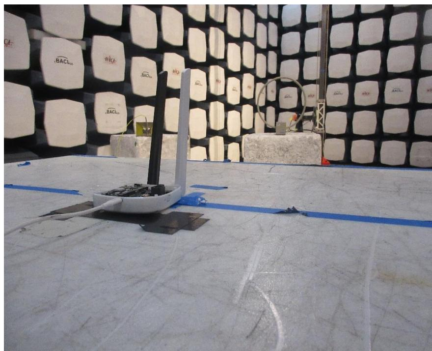
**1.5 Radiated Spurious Emissions: 30MHz - 1GHz Front View at 3 meters**
