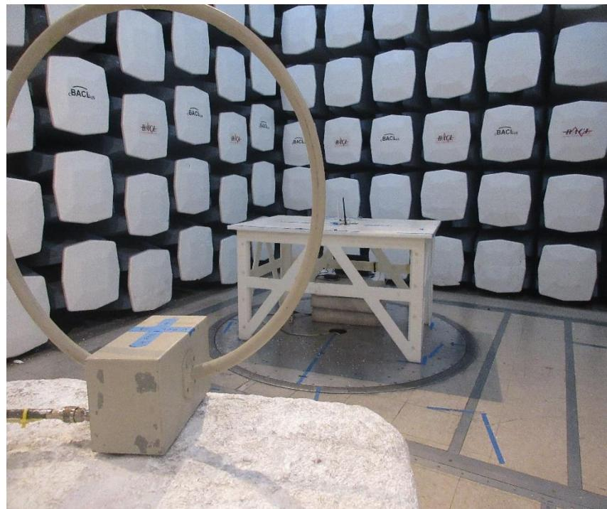
**1.4 Radiated Spurious Emissions: 9 kHz – 30 MHz, Perpendicular Rear View at 3 meters**
