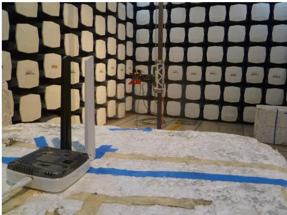
**1.9 Radiated Spurious Emissions: 18-26.5 GHz Front View at 3 meter**
