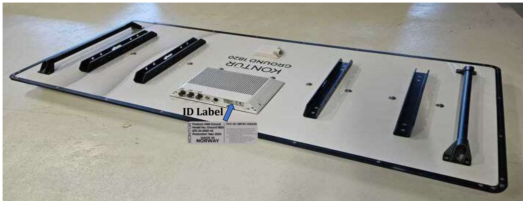
Figure 1: Label placement antenna
